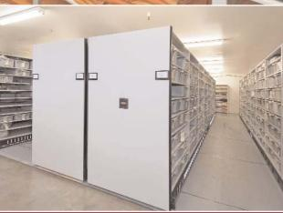
A mechanical-assist mobile system (top) houses bulk property formerly in satellite storage. Stationary shelving (center) keeps inmate-issue clothing organized. The powered mobile system (bottom) doubled storage capacity for inmate property. in satellite storage and only accessible through doors that people in other departments had to open and close.
